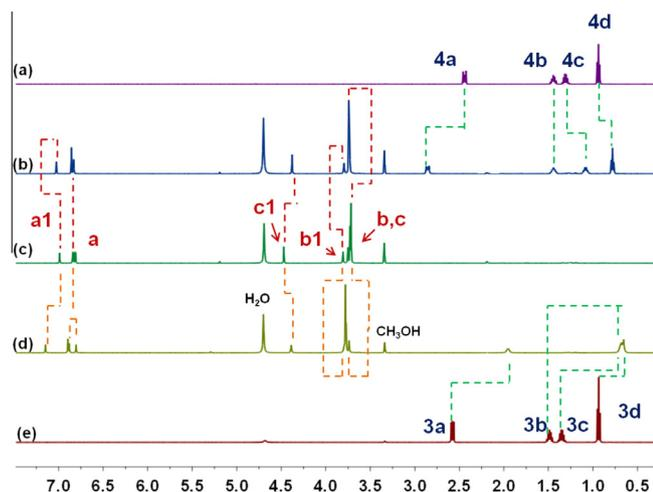
**Figure 1.**  $^1\text{H}$  NMR spectra (500 MHz, chloroform-*d*/methanol-*d*<sub>4</sub> = 1:1, 295 K): (a) G4 (5.00 mM); (b) **H** (5.00 mM) and G4 (5.00 mM); (c) **H** (5.00 mM); (d) **H** (5.00 mM) and G3 (5.00 mM); and (e) G3 (5.00 mM).
