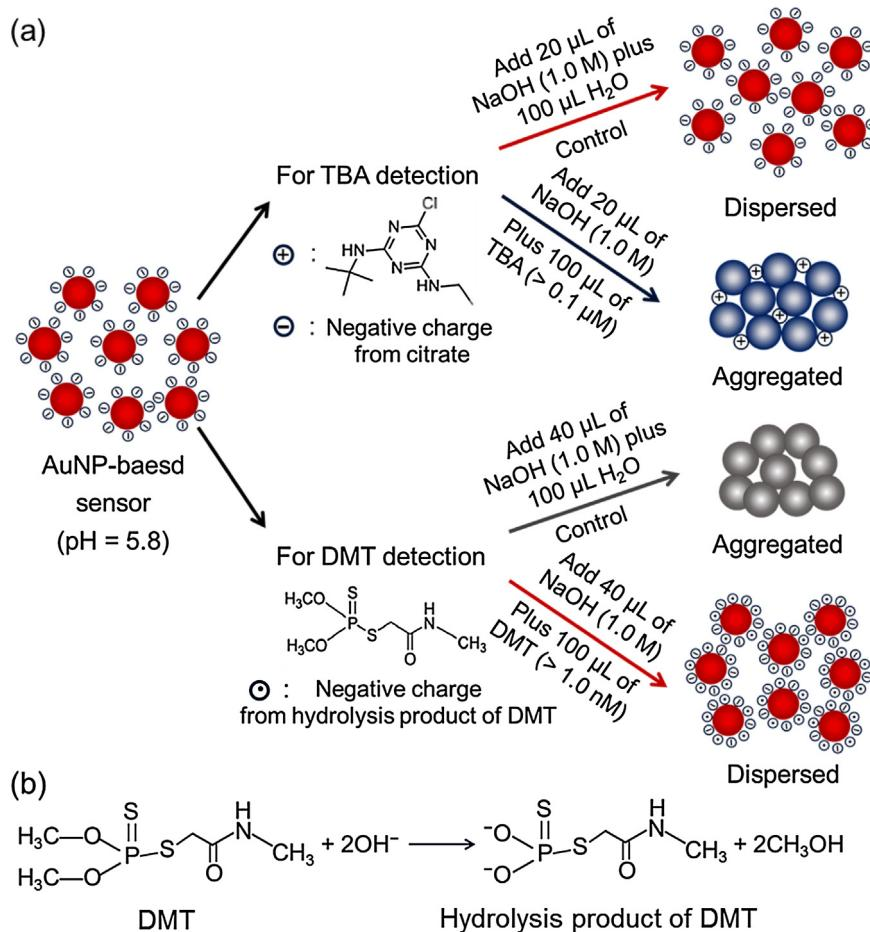
**Scheme 1.** (a): Schematic illustration of the mechanisms of the AuNP-based colorimetric sensor for rapid pesticide residue detection of terbutylazine (TBA) and dimethoate (DMT); (b): Reaction equation of the DMT at alkaline conditions.
